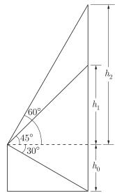
$$\begin{split} \tan 30^\circ &= \frac{h_0}{300}; \; h_0 = 300 \tan 30^\circ \\ &= \frac{300}{\sqrt{3}} m \; = 100 \sqrt{3} \\ \tan 45^\circ &= \frac{h_1}{300}; \; h_1 = 300 \tan 45^\circ = 300 \; m \end{split}$$
