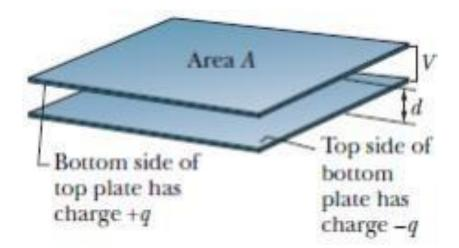
This conventional arrangement, called a parallel-plate capacitor, consisting of two parallel conducting plates of area A separated by a distance d.
