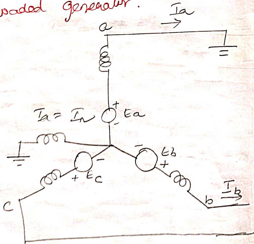
Circuit diagram of single  $I_a$  LG fault on phase a of an unloaded generator.
