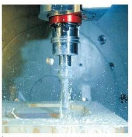
Since Zerodur is one of the most expensive materials in the world, technologies, such as ultrasonic machining, are used to prevent a part from turning into scrap by loose tolerances
