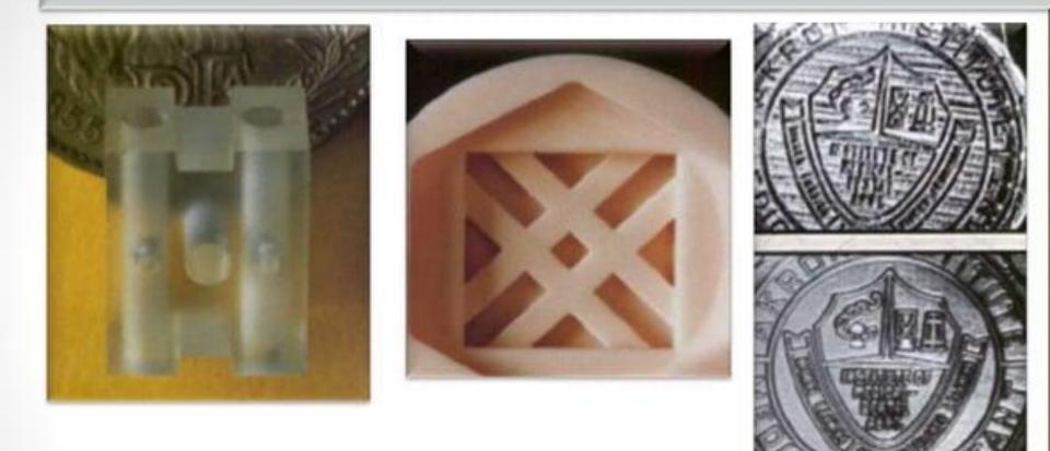
1- The first picture on the left is a plastic sample that has inner grooves that are machined using USM.
