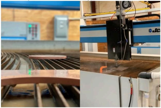
We have a fully contained water jet cutting system that is environmentally friendly, capturing spent garnet and recycling the process water rather than dumping it down the drain.
