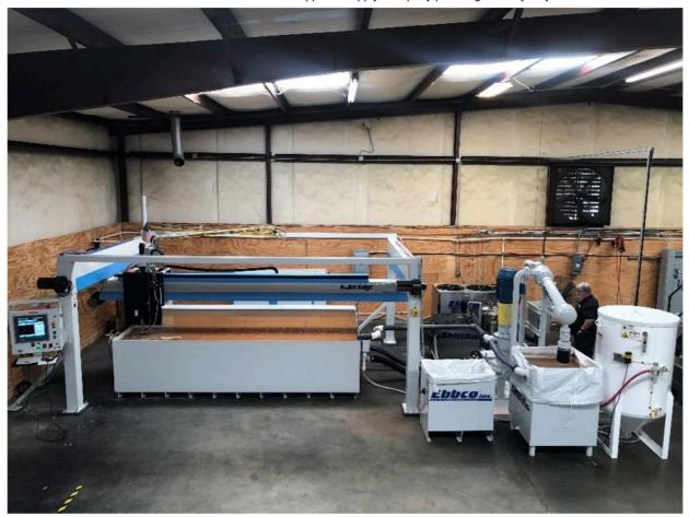
The high rail motion system opens up the cutting envelope for easy access. SCS utilizes a single 3-axis abrasive cutting head, with 12" of Z travel. Several productivity enhancements were added including lights out cutting and IGEMS nesting software. An abrasive removal system and closed loop filtration system combine making this a fully contained, environmentally friendly waterjet system.
