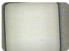
Fig 1.8 A UM-machined square hole in 0.0175-in. thick glass. The machined feature exhibits a clean edge, and the natural corner radius is < 0.005 in.
