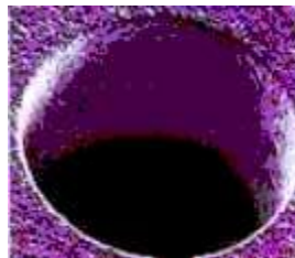
Fig 1.12 SEM of a 0.64mm hole ultrasonically machined in an alumina substrate
