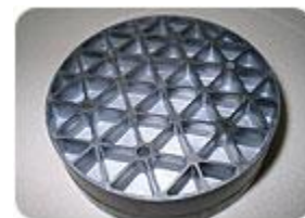
Fig 1.9 Honeycomb structure machined on the back of a silicon mirror for NASA.
