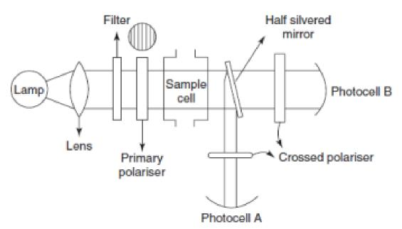
Instrumentation used in nephelometry and turbidimetry is very similar to spectrophotometer devices.
