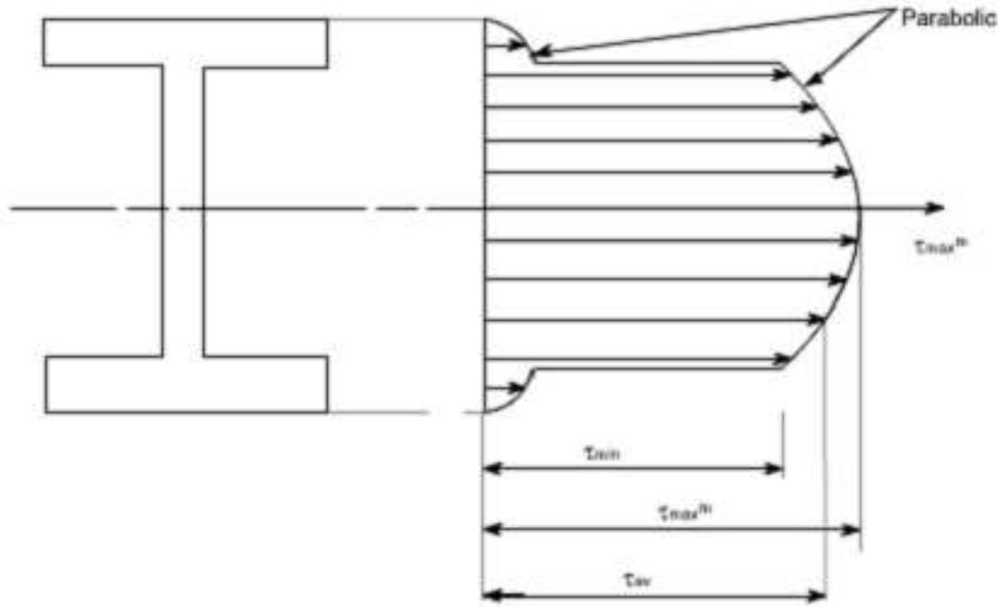
This distribution is known as the “top – hat” distribution. Clearly the web bears the most of the shear stress and bending theory we can say that the flange will bear most of the bending stress.
