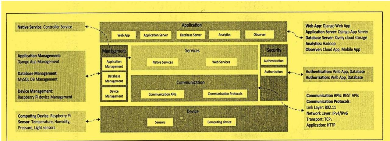
Mapping functional Groups to operational view specifications for the weather monitoring system.
