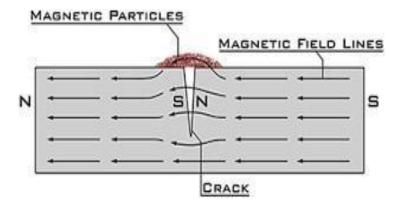
When a bar magnet is broken in the center of its length, two complete bar magnets with magnetic poles on each end of each piece will result. The magnet is just cracked but not broken completely in two, a north and south pole will form at each edge of the crack. The magnetic field exits the north pole and re-enters at the south pole.
