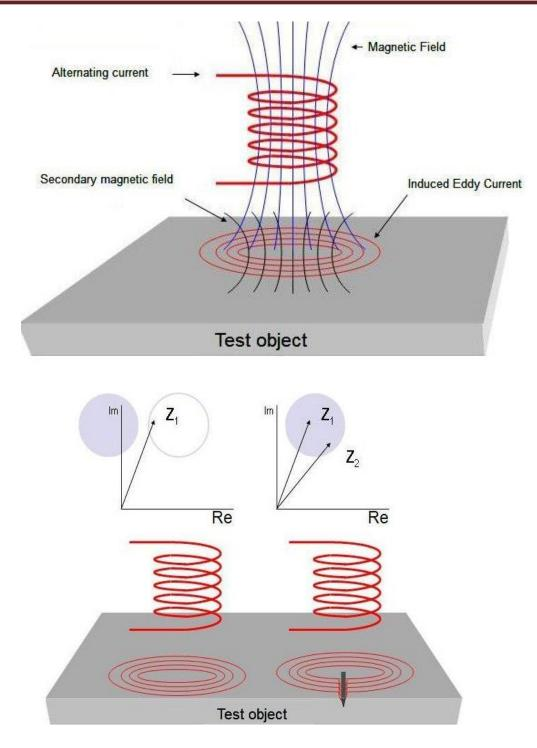
**Uses:** The technology is now widely used in the aerospace, automotive, petrochemical, and power generation industries for the detection of surface or near-surface defects in materials such as aluminum, stainless steel, copper, titanium, brass, Inconel®, and even carbon steel (surface defects only).
