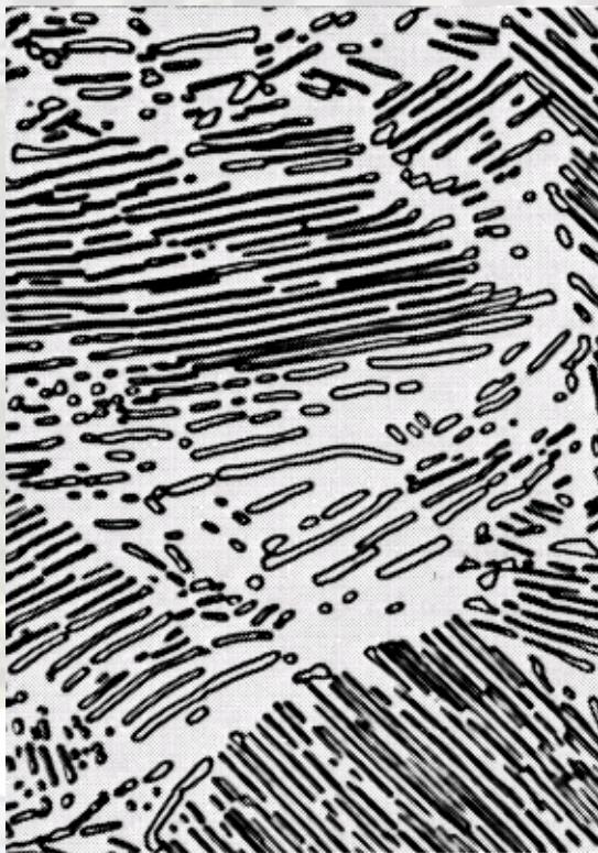
In the micrograph, the dark areas are  $\text{Fe}_3\text{C}$  layers, the light phase is  $\alpha$ - ferrite
