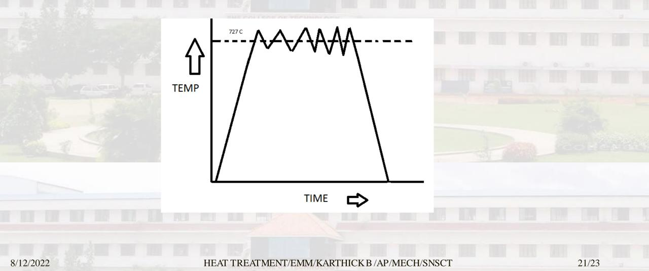
• For tool and high speed steel heating at the temperature range between 750° - 800°C then hold at this temperature and then slow cooling.
