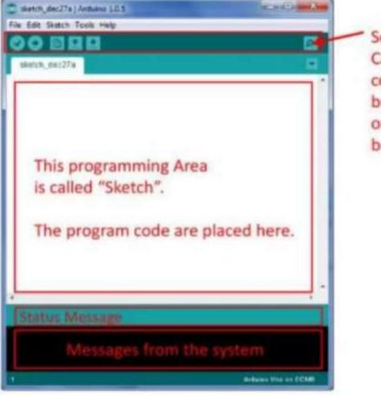
Serial monitor, Can use this to issue commands to the board, and read outputs from the board.
