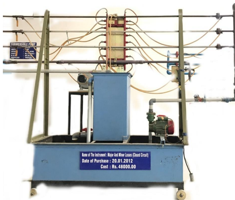
Minor Loss Setup
