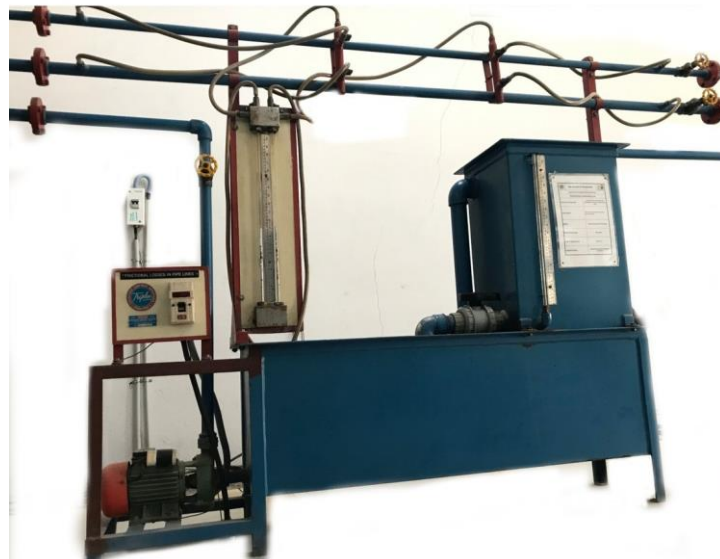
Pipe setup for Friction Factor
