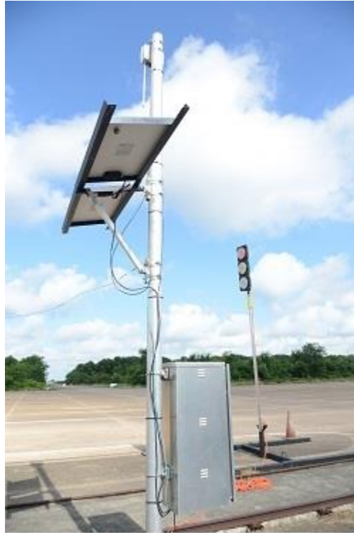
Figure 2. Equipment collecting data from connected vehicles and a traffic signal at a test track.
