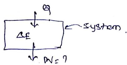
2. A piston and cylinder machine contains a fluid system which passes through a complete cycle of four processes. During a cycle, the sum of all heat transfer is  $-170 \text{ kJ}$ . The system completes 100 cycles per min. Complete the following table showing the method for each item, and compute the net rate of work output in kW.
