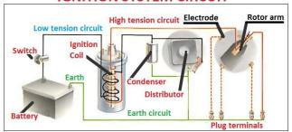
Segment on the distributor cap □> plug leads □> plug caps □> central electrode □> nose of the plug
