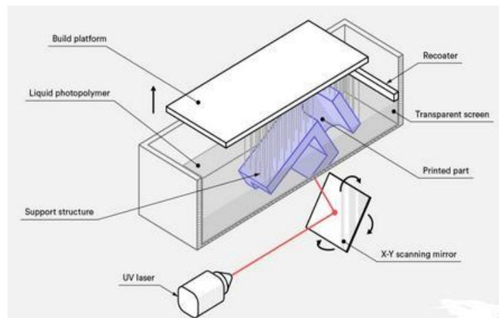
Stereolithography provides advantages in **speed, cost-effectiveness, flexibility, and precision**. These advantages make stereo lithography for medical device design, among many other industries, a vital process for creating models and prototypes that help refine and prove designs.
