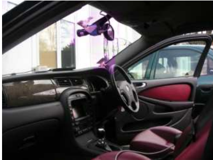
(a) Forward-looking and driver video cameras. The cameras are highlighted.
