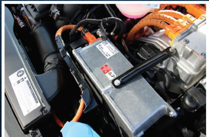
Figure 2.9 Orange high-voltage cables
