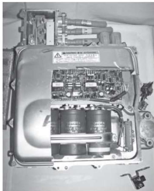
Figure 3-37 The inverter assembly for a Toyota hybrid vehicle.
