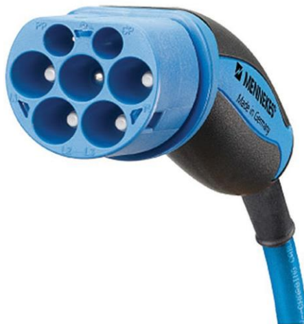
Figure 6.14 Type 2 plug. The pins from the top left and clockwise are: Proximity (PP), Control pilot (CP), Neutral (N), L3, L2, L1 and the Earth pin in the centre (Source: Mennekes)
