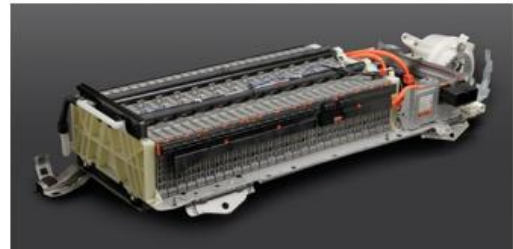
Figure 5.8 Third-generation NiMH battery (Source: Toyota)
