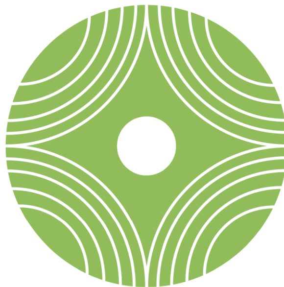
Figure 37. SynRM with axially laminated rotor [23].
