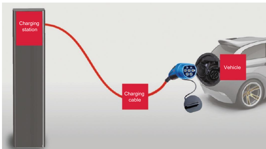
Figure 6.7 Case C: The charging cable is permanently connected to the charging station (Source: Mennekes)
