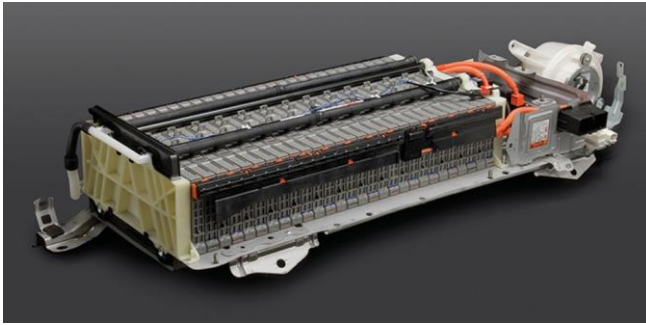
Figure 5.8 Third-generation NiMH battery(Source: Toyota)
