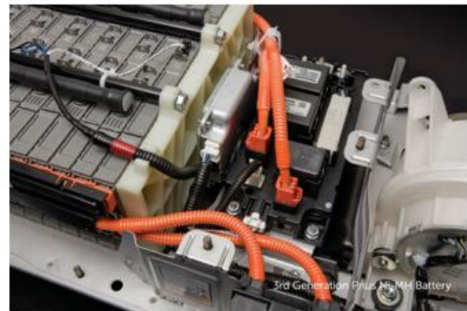
Figure 5.7 Toyota NiMH battery and management components (Source: Toyota)
