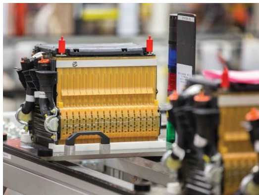
Figure 5.1 Battery pack for the Chevrolet Spark (Source: General Motors)
