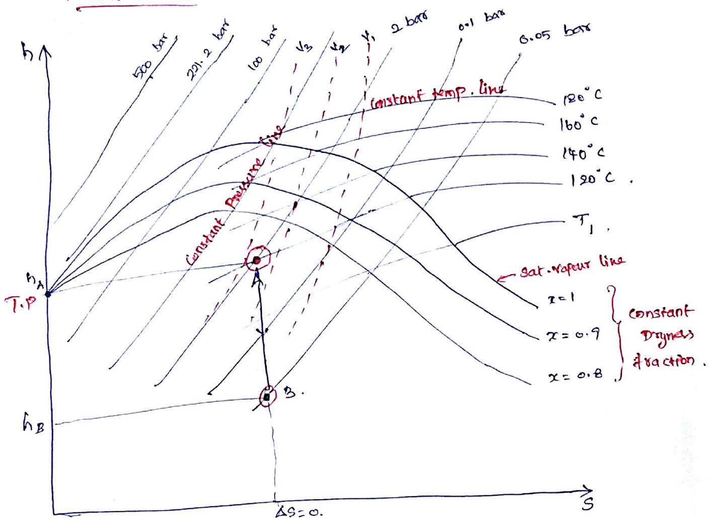
It is used to find out the properties of stream in various condition.
