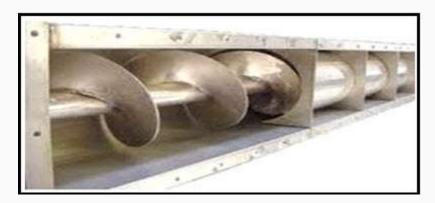
The screw conveyor is generally used to move grains horizontally. However, it can also be used at any angle upto 90° from the horizontal, but the capacity correspondingly reduced as per the inclination of conveyance.
