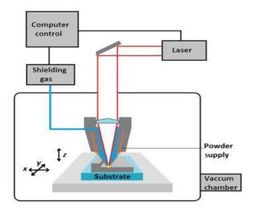
Laser, powder, and laser-powder interaction are common in both LENS and SLS/SLM. The major difference is that the former is blown-powder technique while the latter is powder bed technique. LENS generally uses higher laser power (in terms of kilowatt) and larger spot size, which make its deposition rate higher.
