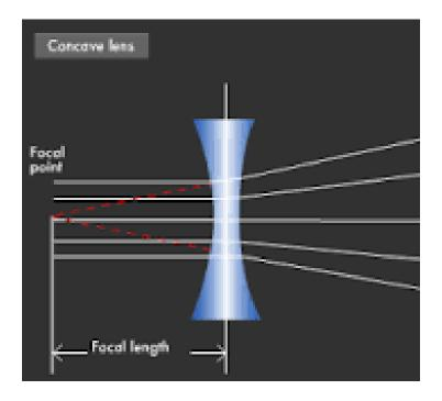
Lenses may be divided broadly into two main types: **convex and concave**. Lenses that are thicker at their centers than at their edges are convex, while those that are thicker around their edges are concave. A light beam passing through a convex lens is focused by the lens on a point on the other side of the lens.
