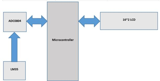
The ADC0804 IC is an 8-bit parallel ADC in the family of the ADC0800 series from National Semiconductor. It works with +5 volts and has a resolution of 8bits. The step size and Vin range varies for different values of Vref/2.
