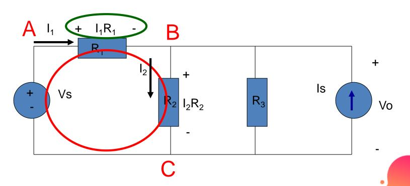
Starting at node A, add the 1st voltage drop: + I<sub>1</sub>R<sub>1</sub>
