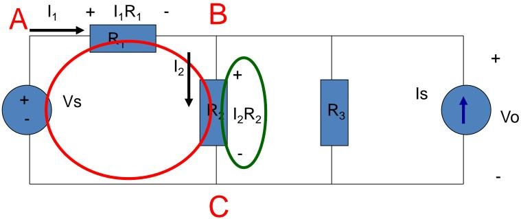
Add the voltage drop from B to C through  $R_2$ :  $+ I_1R_1 + I_2R_2$
