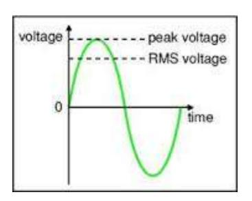
Parameters V and I are in sine wave.
