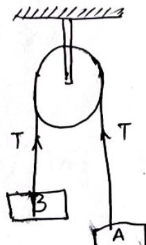
The string is passing through smooth pulley and hence tension on each side of the string will be equal.
