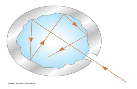
When heated, it would emit more radiations from a unit area through the hole at a given temperature => *perfect emitter*
