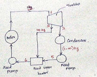
The steam expands from condition 1 through the turbine. At the pressure corresponding to point 2, a quantity of steam with m kg per kg of steam supplied from beilers is bled off for heating feed water. The rest of steam (1-m) kg Completes the expansion and is exchausted to the Condenser pressure P3. The amount of steam is then Condensed and pumped to the Same pressure as the bleed steam. The bleed steam of m kg and feed water are mixed in the feed water under
