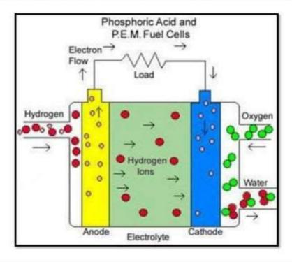
Molten phosphoric acid is the electrolyte used in this type of fuel cell. It operates at high temperature up to 200 degree Celsius. It has an efficiency of up to 55%. This type of fuel cell is most commonly used in commercial cars.
