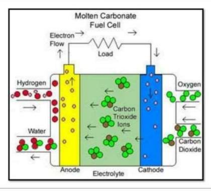
Molten alkaline carbonate like sodium bicarbonate is used as the electrolyte. They can produce high powers up to 100 Mega Watts. Thus they can be used as high power generators. They can also be operated at high temperatures up to 650 degree Celsius. They are not so expensive in production and hence can be used for commercial uses. It has an efficiency of almost 55%.
