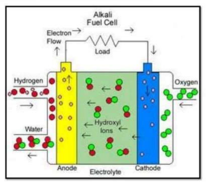
This type of fuel cell was been introduced in the early 1960's. As the electrolyte used for this device is aqueous alkaline solution like potassium hydroxide, the procedure for electricity consumption is rather expensive.
