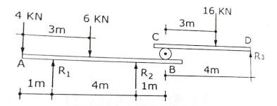
4. Find the support reactions of the beam shown of the beam shown
