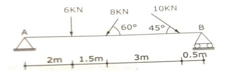
5. Find the support reactions of the beam shown of the beam shown
