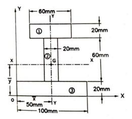
4. Find the Moment of inertia of the given section shown in diagram about the horizontal axes.
