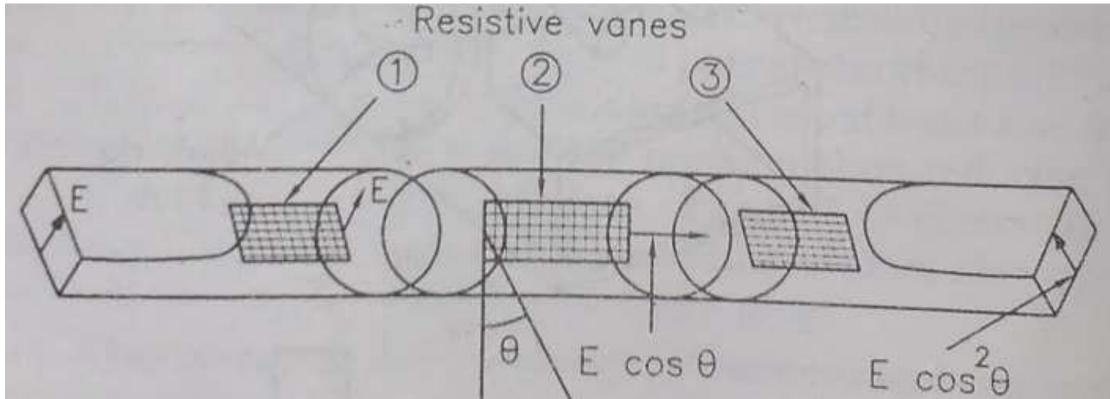
The vane positioned at center of guide can be moved laterally from center, where it provides maximum attenuation to the edges where the attenuation is considerably reduced since E lines are always concentrated at the center of waveguide.
