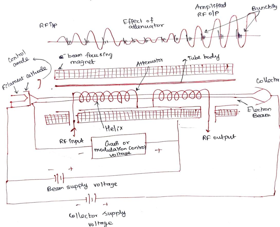
\* - During transit along the axis, the electron beam transfers great amount of energy to the traveling signal wave and thus signal field amplitude increases.
