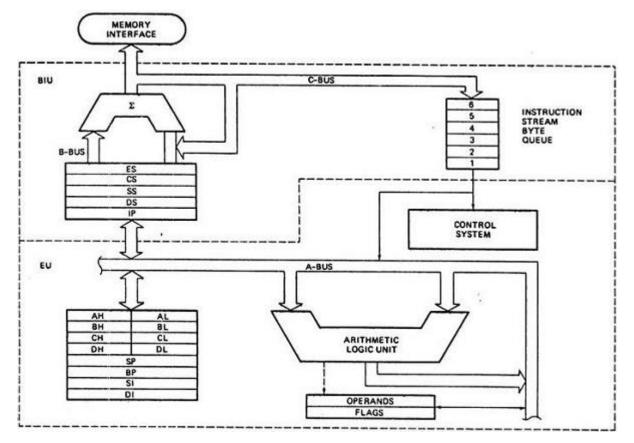
8086 Microprocessor is divided into two functional units, i.e., EU (Execution Unit) and BIU (Bus Interface Unit).
