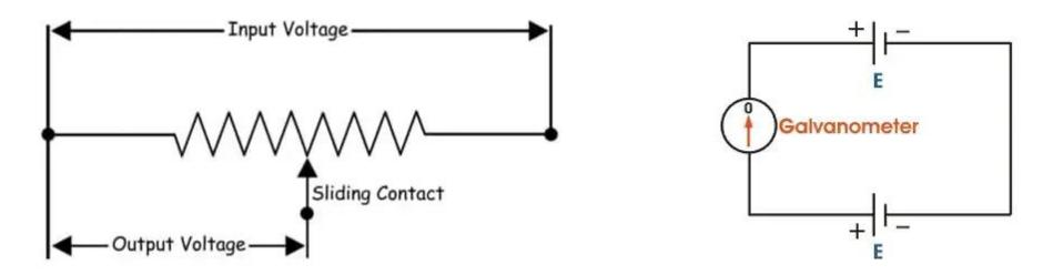
A potentiometer has the two terminals of the input source fixed to the end of the resistor. To adjust the output voltage the sliding contact gets moved along the resistor on the output side.
