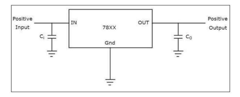
• The input capacitor C is used to prevent unwanted oscillations and the output capacitor, C acts as a line filter to improve transient response
