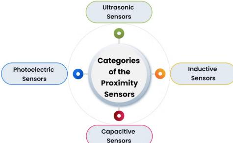
Proximity sensors detect the presence or absence of objects near the sensor without physical contact. They often emit a beam of radiation like infrared or an electromagnetic field. They can be used for process monitoring and control, object counting, assembly lines, and determining available space. Proximity sensors are common in retail settings, industrial complexes, and parking lots. Some examples are photoelectric, magnetic, capacitive, inductive, and ultrasonic.
