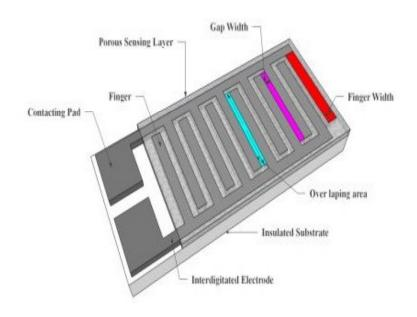
These sensors are used to track the air's relative humidity, or the percentage of water vapour and other gases present in the air.
