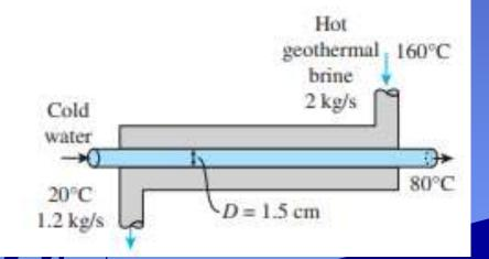
$C_h = \dot{m}_h c_{ph} = (2 \text{ kg/s})(4.31 \text{ kJ/kg} \cdot \text{K}) = 8.62 \text{ kW/K}$  $C_c = \dot{m}_c c_{pc} = (1.2 \text{ kg/s})(4.18 \text{ kJ/kg} \cdot \text{K}) = 5.02 \text{ kW/K}$
