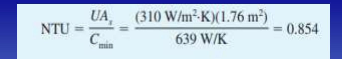
The effectiveness of this heat exchanger corresponding to c = 0.764 and NTU = 0.854 is (from the chart c)
