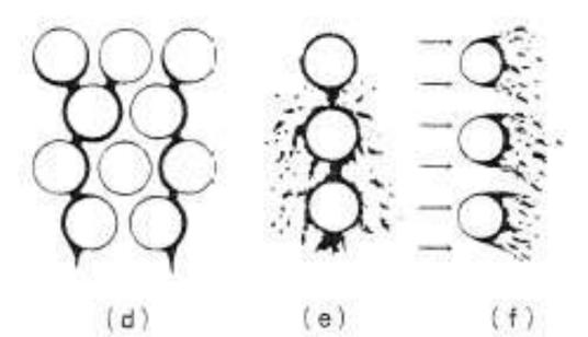
Figure 1. Modes of condensate inundation in horizontal tube banks.
