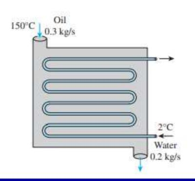
$$C_{h} = \dot{m}_{h}c_{ph} = (0.3 \text{ kg/s})(2.13 \text{ kJ/kg} \cdot ^{\circ}\text{C}) = 0.639 \text{ kW/K}$$
