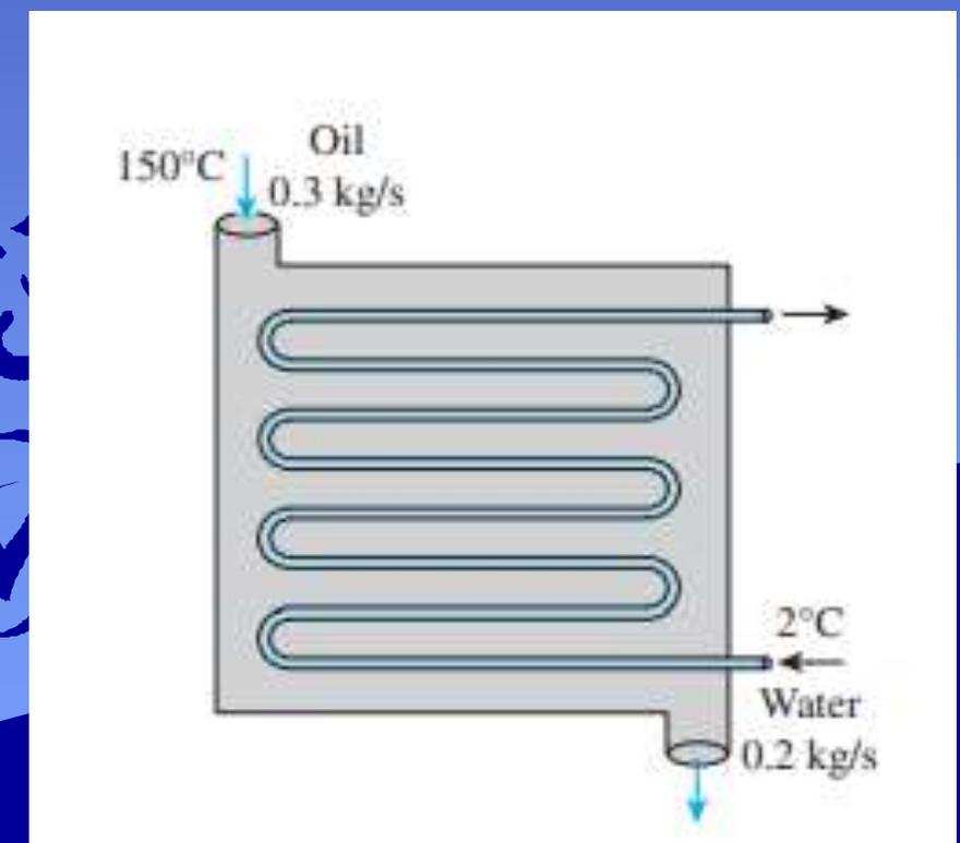
$$C_h = \dot{m}_h c_{ph} = (0.3 \text{ kg/s})(2.13 \text{ kJ/kg}\cdot^\circ\text{C}) = 0.639 \text{ kW/K}$$
