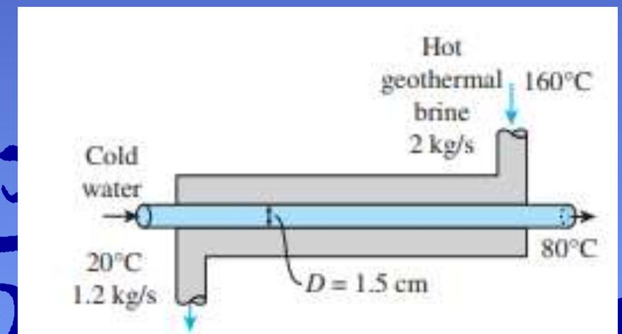
$$C_h = \dot{m}_h c_{ph} = (2 \text{ kg/s})(4.31 \text{ kJ/kg}\cdot\text{K}) = 8.62 \text{ kW/K}$$
