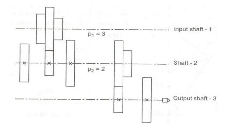
Example.4.4.A nine speed gear box, used as a head stock gear box for a turret lathe, is to provide a speed range of 180 rpm to 1800 rpm. Using atandard step ratio draw the speed diagram, and kinematic layout.
