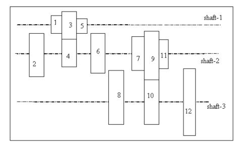
Example.4.4. Design the layout of a 12 speed gear box for a lathe the minimum and maximum speeds are 100 rpm and 1200 rpm. Power is 5kw from 1440 rpm induction motor. Construct a speed diagram using a standard speed ratio. Calculate the number of teeth in each gear wheel and sketch the arrangement of gear box.
