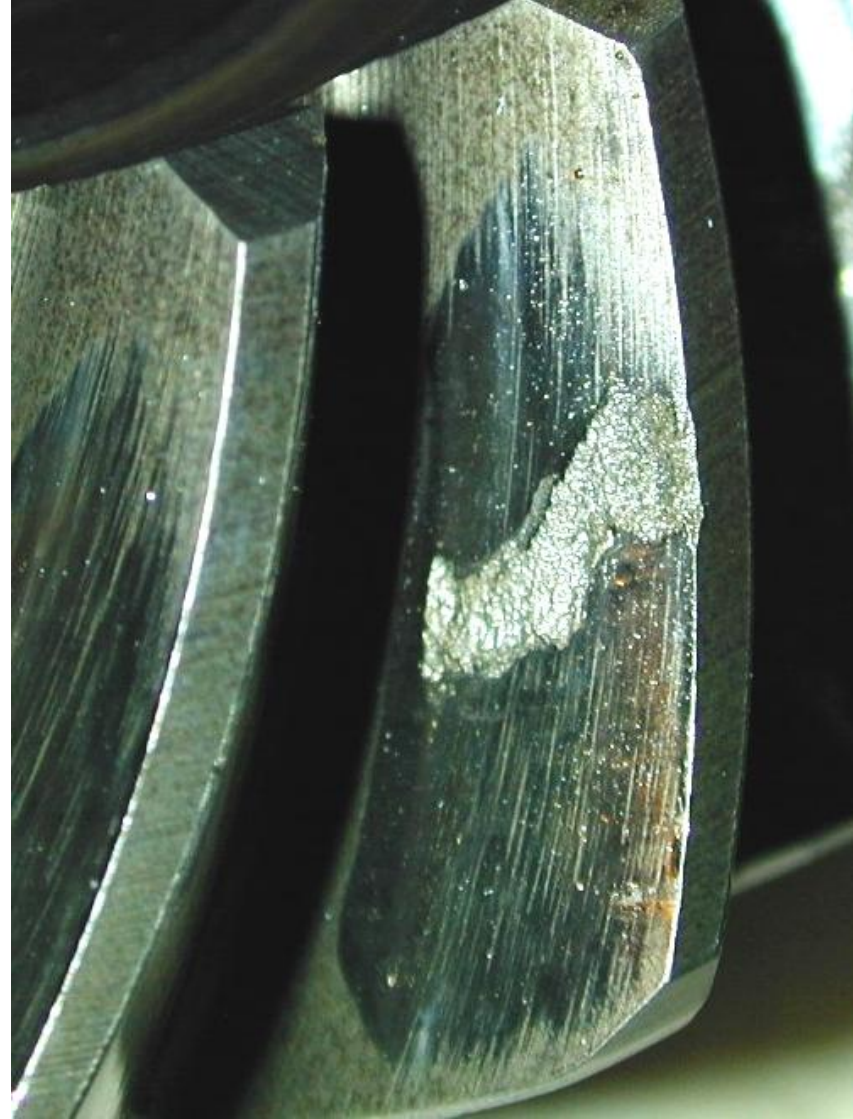
Figure 3. Fatigue Crack in Gear Tooth Root Fillet.
