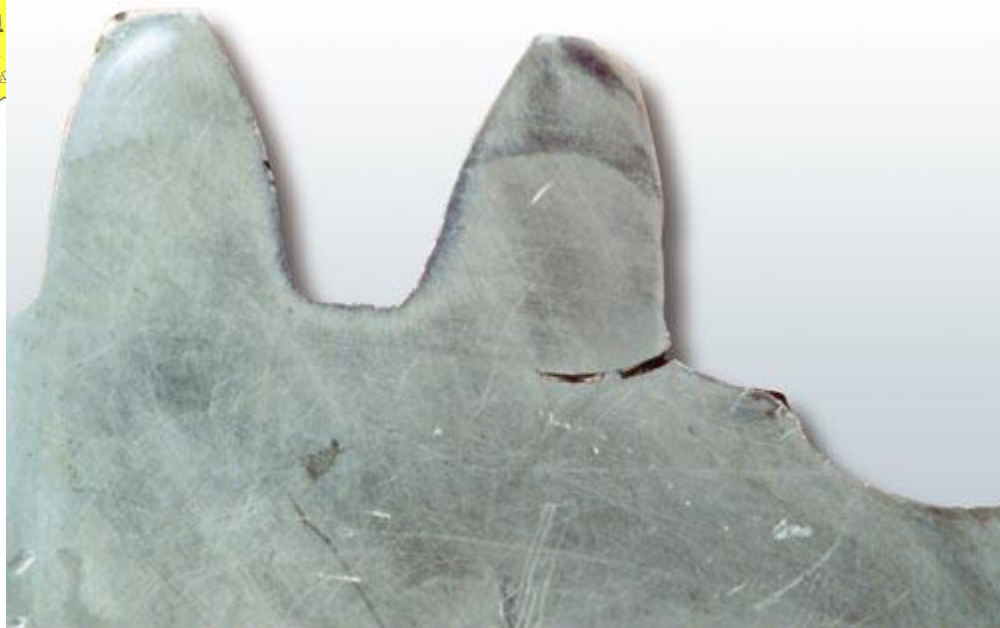
Figure 3. Fatigue Crack in Gear Tooth Root Fillet.
