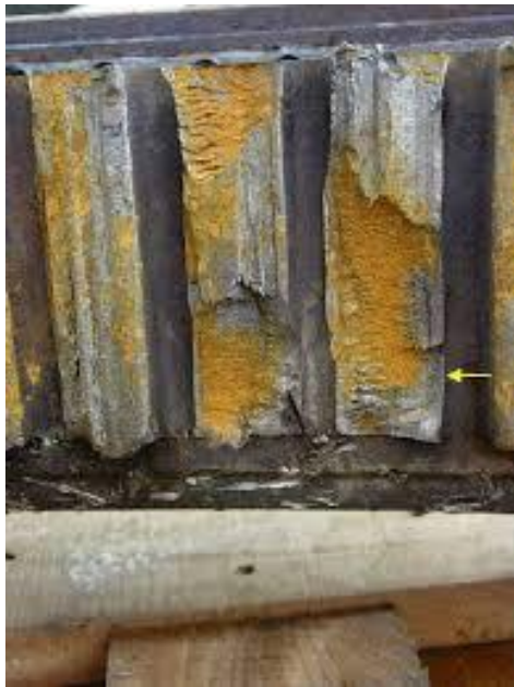
Figure 3. Fatigue Crack in Gear Tooth Root Fillet.
