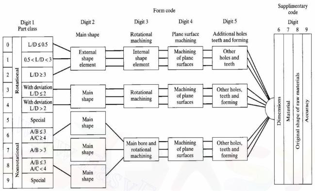
The optiz coding is most likely the best-known coding system. It was developed by H. optiz of the Aachen Tech University in West Germany. The code uses a hybrid structure. However, except the first digit, it resembles a chain structure more closely. It has following advantages over the existing system
