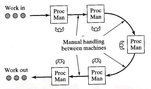
Machine cell with manual handling between machines. Shown is a If-shaped machine layout. (Key: "Proc" 0= processing Operation (e.g., mill. turn, etc.), "Man" = manual operation; arrows indicate work flow.)
