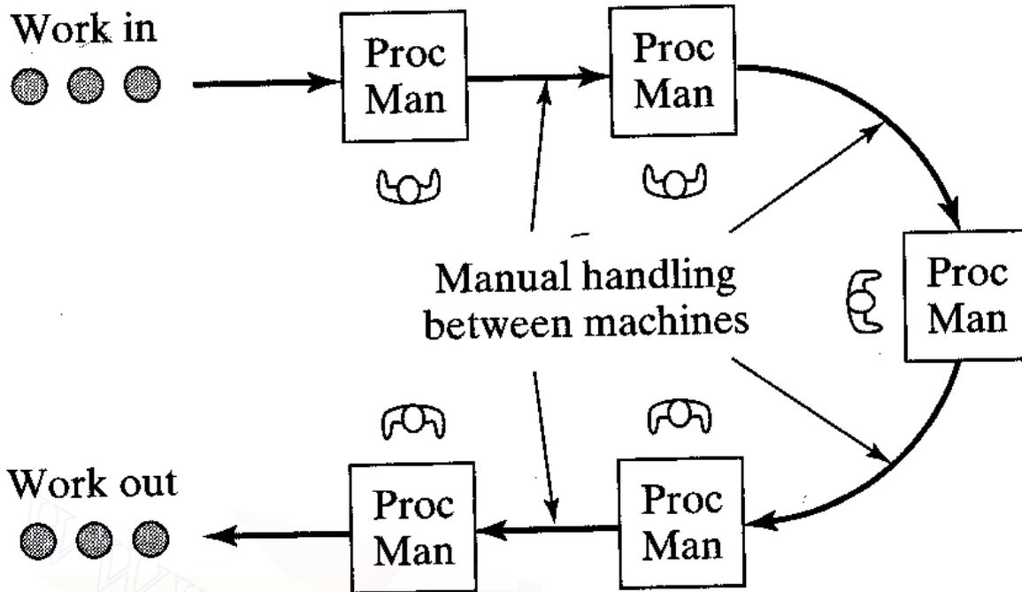
Machine cell with manual handling between machines. Shown is a If-shaped machine layout. (Key: "Proc" = processing Operation (e.g., mill. turn, etc.), "Man" = manual operation; arrows indicate work flow.)
