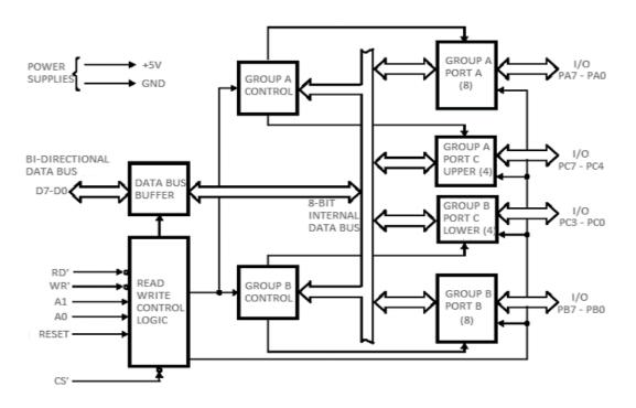
It consists of 40 pins and operates in +5V regulated power supply. Port C is further divided into two 4-bit ports i.e. port C lower and port C upper and port C can work in either BSR (bit set rest) mode or in mode 0 of input-output mode of 8255. Port B can work in either mode 0 or in mode 1 of input-output mode. Port A can work either in mode 0, mode 1 or mode 2 of input-output mode.
