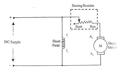
The connection diagram shows the method of connecting starting resistor in the armature circuit during starting. During starting, the movable arm of starting resistor is in the position. When the motor attains rated speed the movable arm is placed in the other end (Resistance, R = 0)
