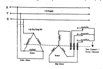
The addition of rotor resistance enables slip ring Induction motor to develop a high starting torque. Hence such motors can be started under heavy load.
