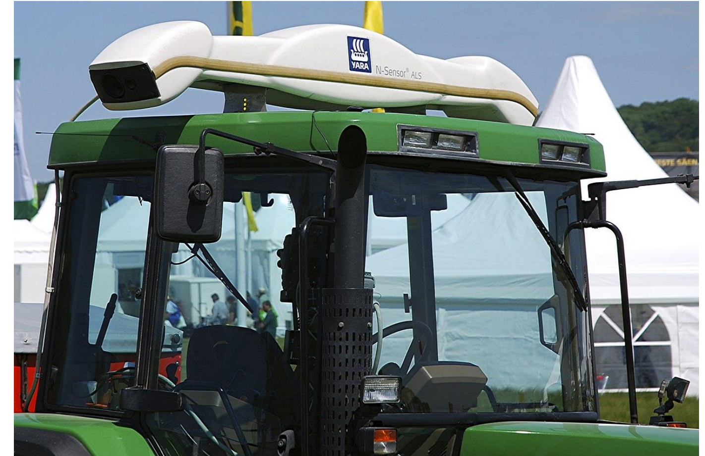
Yara N-Sensor ALS mounted on a tractor's canopy – a system that records light reflection of crops, calculates fertilisation recommendations and then varies the amount of fertilizer spread
