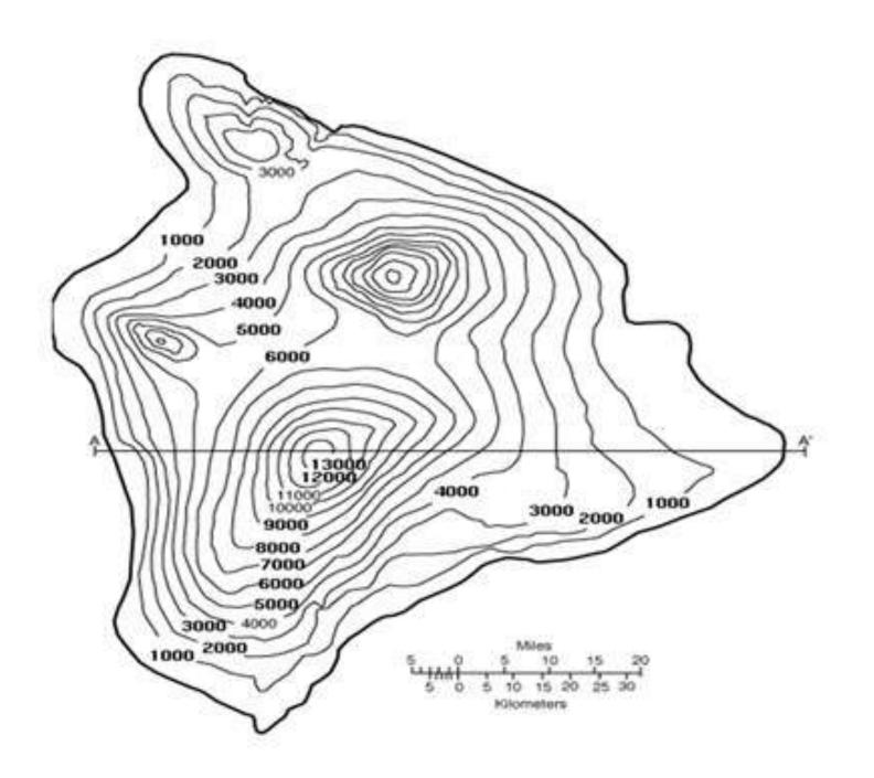
Topographic maps; for example, have a scale of 1:24,000 (which means that one inch measured on the map represents 24,000 inches (2000 feet) on the ground).
